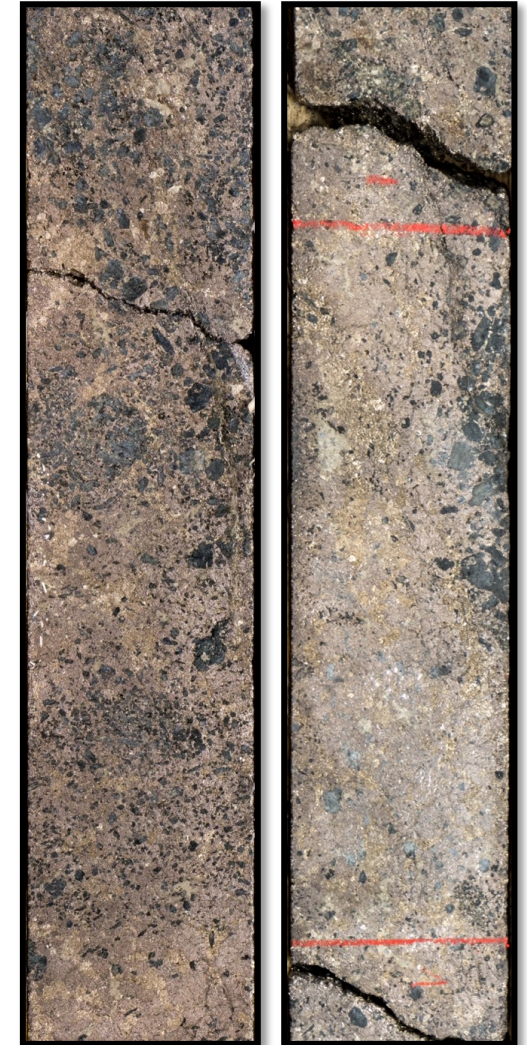
Hole NBI-24-001 - Massive pyrrhotite-pentlandite with coarse grained pentlandite and minor stringers of chalcopyrite, from a 1.36 m sample that returned 8.08% Ni, 0.19% Co, 0.23% Cu, and 0.85 g/t Pt+Pd
